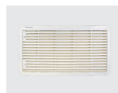
LS300 vent and frame cut out required W490 mm x H249 mm. Each vent has open area of 667 cm 2
