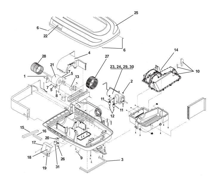
Only Parts Identified With An Index Number Are Available For Service Replacement.
